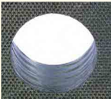
hole exit in CFRP with woven cover layer hole D=6.35 mm
